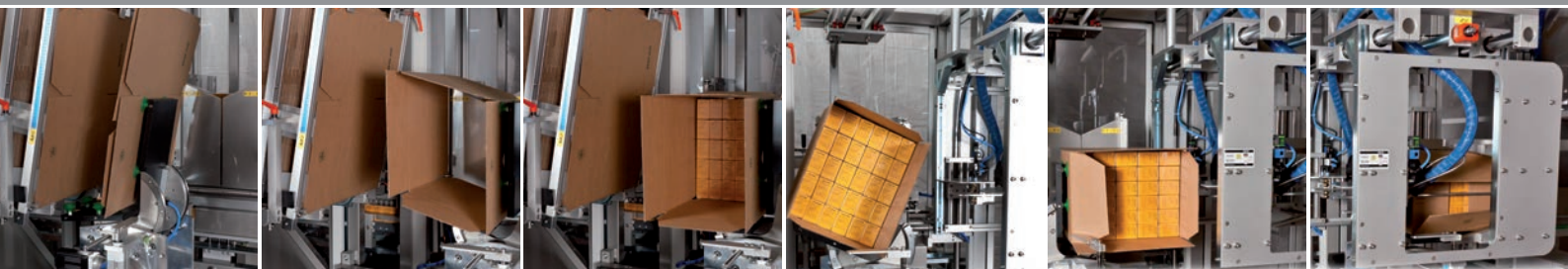
» Case removal from magazine » Case erection » Case filling in upright and horizontal position » Case tilted 90° » Case transfer to sealing unit » Gluing and pressing (Opt: self-adhesive band)
